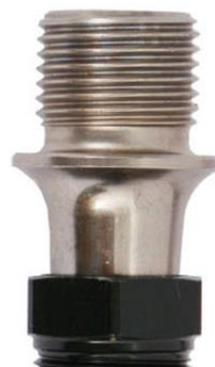
Make sure you are fitting the pedals to the correct side; you can identify them by the orientation of the thread as shown above. Never try to force your pedals to fit, only fasten them using finger tension until you are sure the threads are correctly aligned. Tighten your pedals to the correct tension with a pedal spanner/Allen key before riding your bike.
