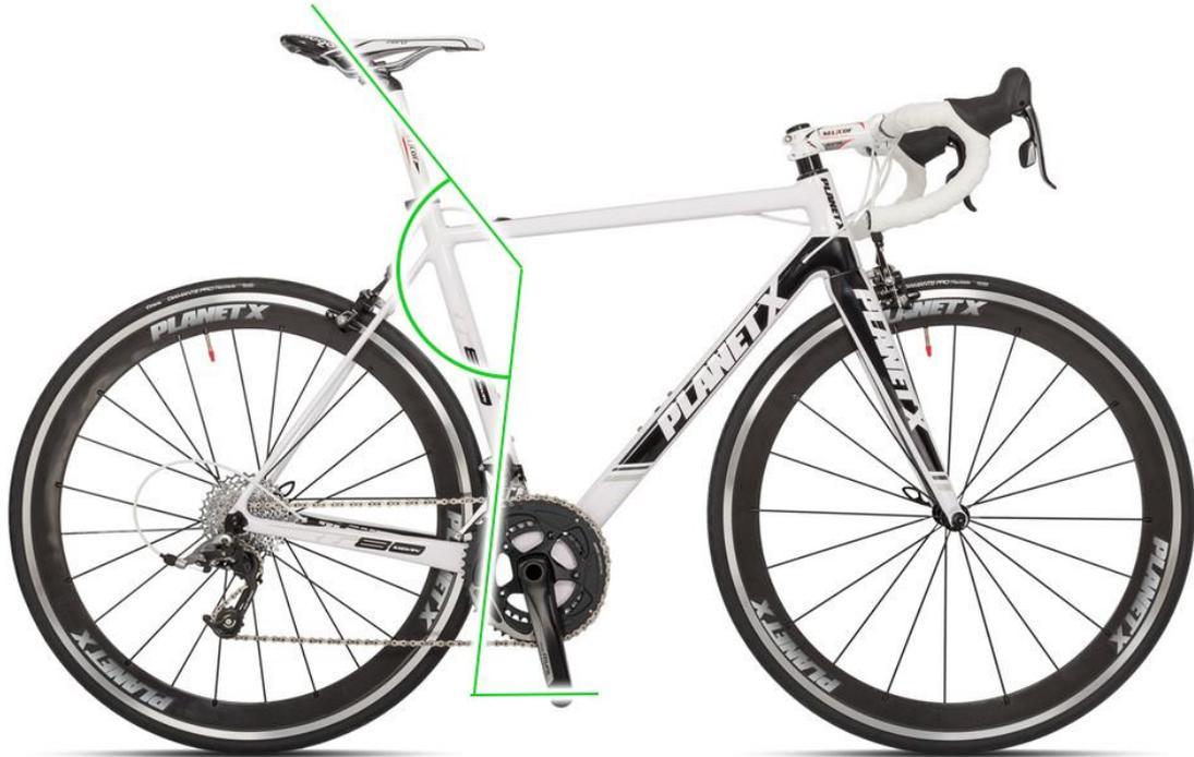
Set your saddle height for the most comfortable riding position. A good starting point is to retain a few degrees of bend at the knee when the pedal is at the lowest possible point.
